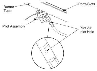
Figure 34 - Pilot Inlet Air Hole
